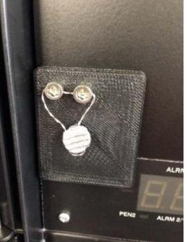
Open the door to the Chart Recorder. Locate the Program/Run Switch. Remove the Wire Lockable Screws. Place the Cover over the Program/Run Switch and align with the threaded holes on the Chart Recorder. Insert the Wire Lockable Screws. Install the Regulatory Seal.
