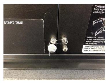
Open the door to the Chart Recorder. Locate the Wire Lockable Screws. Install the Regulatory Seal
