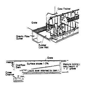
Figure 1. Side Cross Section of a Gravity Flow Gutter
