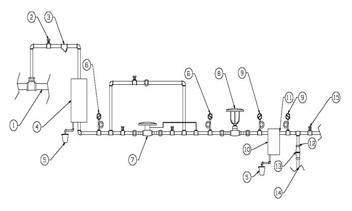
Figure 49. Culinary Steam Piping Assembly for Steam Infusion or Injection
