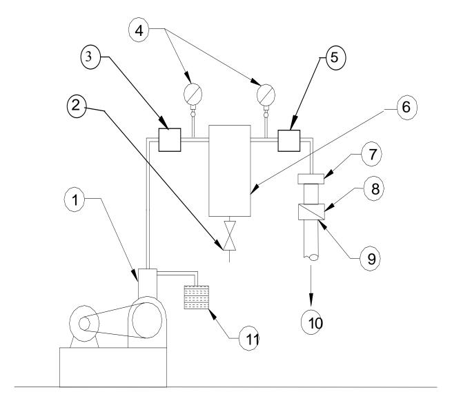
Figure 44. Individual Compression-Type Air Supply
