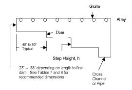
Figure 2. Stepped Gravity Flow Gutter
