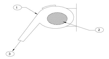
Figure 47. Individual Fan-Type Air Supply
