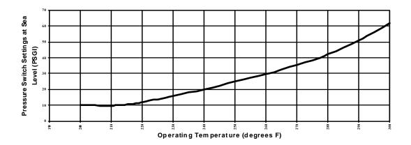
Figure 57. Pressure Switch Setting
