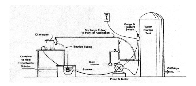
Figure 30. Positive Displacement Chlorinator
