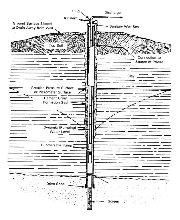
Figure 14. Drilled Well with Submersible Pump
