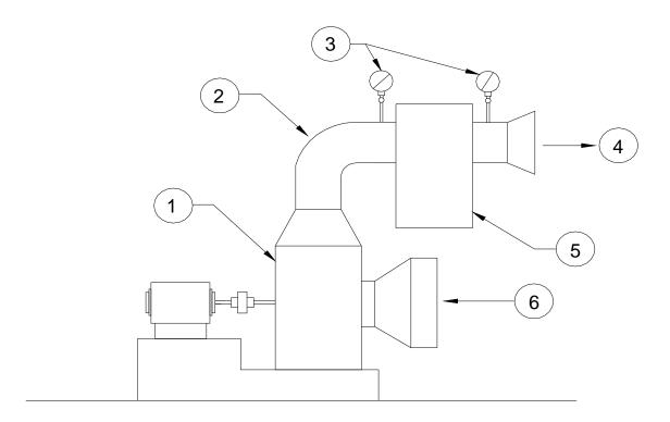
Figure 46. Individual Blower-Type Air Supply
