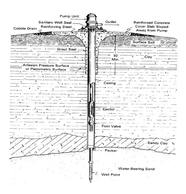
Figure 13. Bored Well with Driven Well Point
