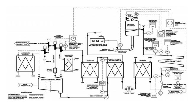
Figure 41. HHST Pasteurizer Utilizing Steam Injection Heating, Vacuum Flash Cooling and a Flow-Diversion Device Located Downstream of the Cooler Section
