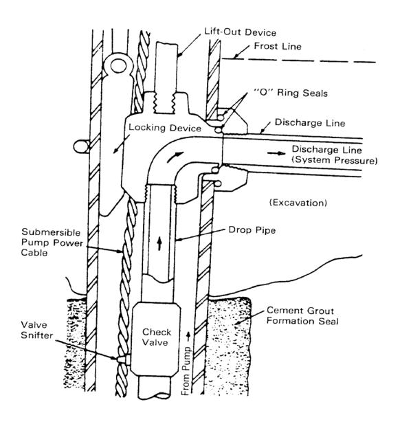
Figure 23. Clamp-on Pit-less Adapter with Concentric External Piping for "Shallow Well"
