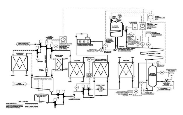
Figure 42. HHST Pasteurizer Utilizing Direct Culinary Steam Infusion and Vacuum Flash Cooling with a Homogenizer Located Downstream
