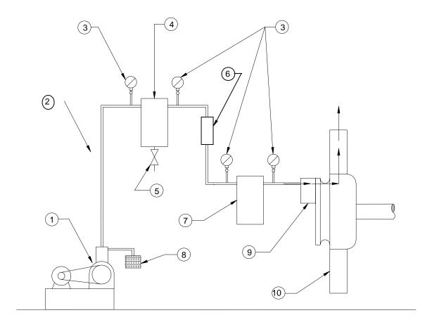
Figure 48. Rotating Mandrel Assembly
