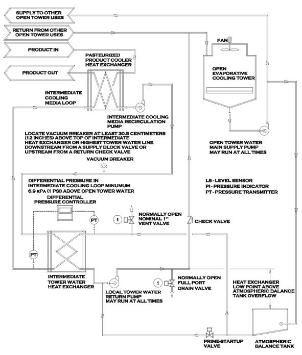
THIS VALVE MUST AUTOMATICALLY OPEN AND REMAIN OPEN WHENEVER THE REQUIRED PRESSURE DIFFERENTIAL IN THE INTERMEDIATE TOWER WATER HEAT EXCHANGER DOES NOT EXIST.
