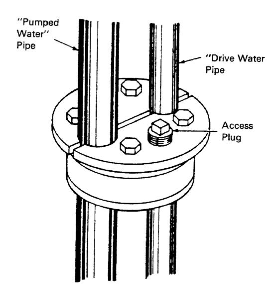
Figure 26. Well Seal for Jet Pump Installation
