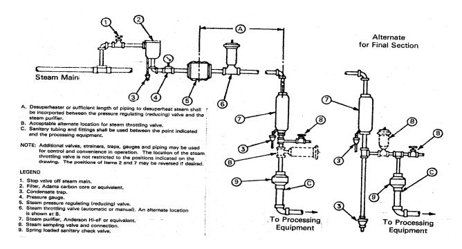
Figure 50. Culinary Steam Piping Assembly for Steam Infusion or Injection (Optional Configuration)
