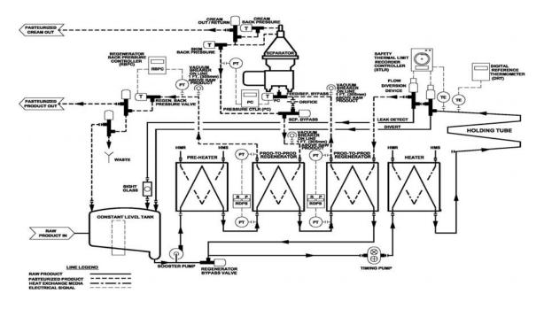
Figure 34. HTST Pasteurizer with a Booster Pump, Timing Pump and a CIP-Type Separator Located Between Two Pasteurized Product Regenerators with a Pre-Heater
