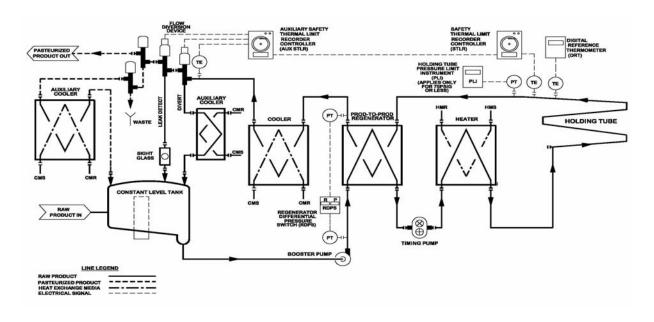
Figure 40. HHST Pasteurizer with a Flow-Diversion Device Located Downstream of the Cooling Section
