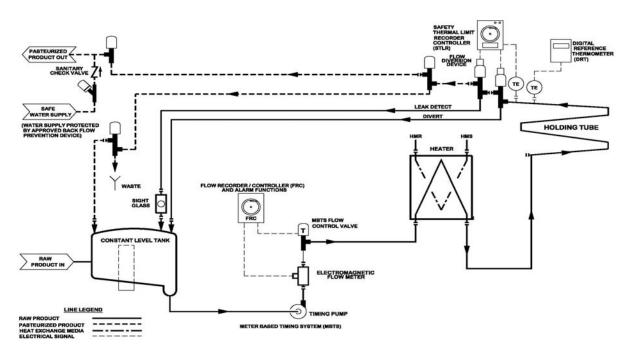
Figure 38. HTST Pasteurizer, without a Regenerator or Cooler Section, with a Meter Based Timing System Located Upstream from an Evaporator
