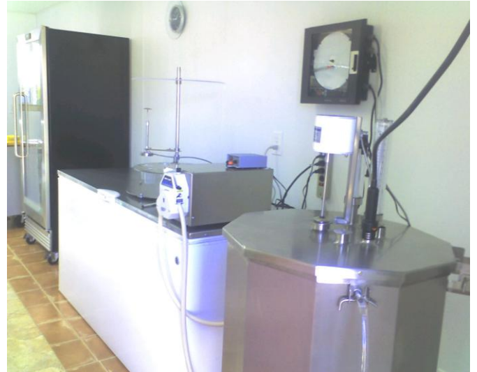
Typical Installation – Pasteurizer, Pump, Packager, Chiller
