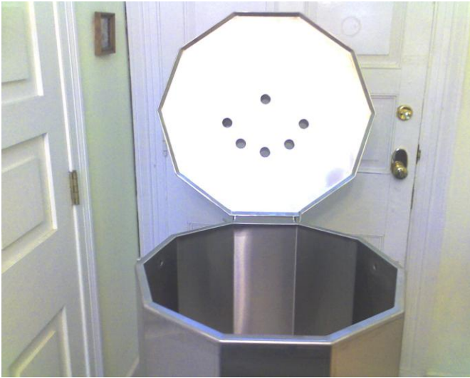
Pasteurizer with lid open to show water jacket and immersion heater in water jacket. Water Jacket is insulated.
