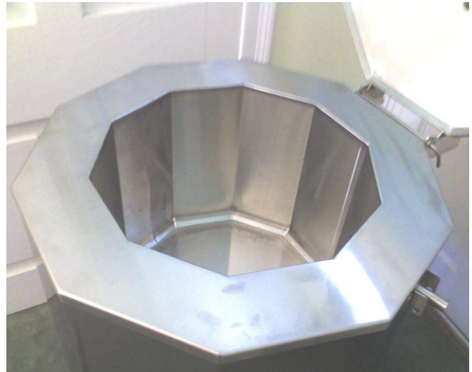
Product Liner – Decagonal shape allows excellent thermal mixing and good cleanability as all angles are greater than 135 degrees
