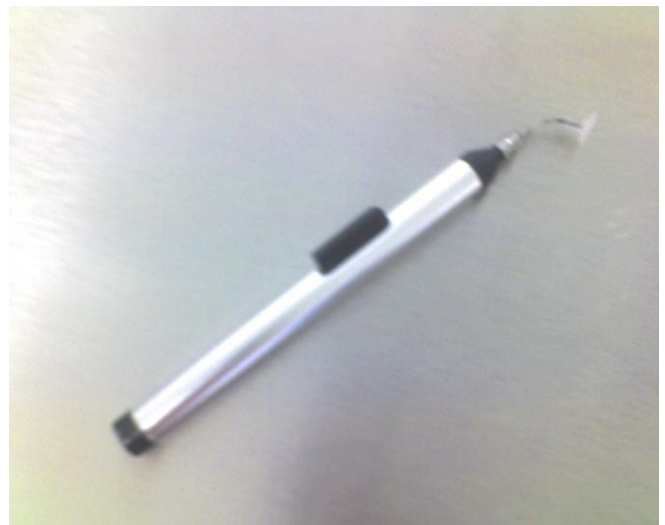
Vacuum pencil to position caps and seals on containers. (Vacuum pencils are typically used in labs to manipulate slides and slide covers and in clean room electronics fabrication to place integrated circuits and chips)
