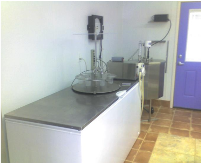
Typical Installation – Pasteurizer, Pump, Packager, Chiller
