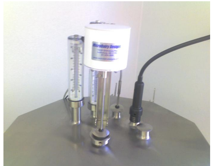
Pasteurizer lid (insulated). Ports included for airspace and product indicating thermometers, chart recorder probe, airspace heater, agitator and for filling/emptying the vat. Lid can be removed for manual cleaning.
