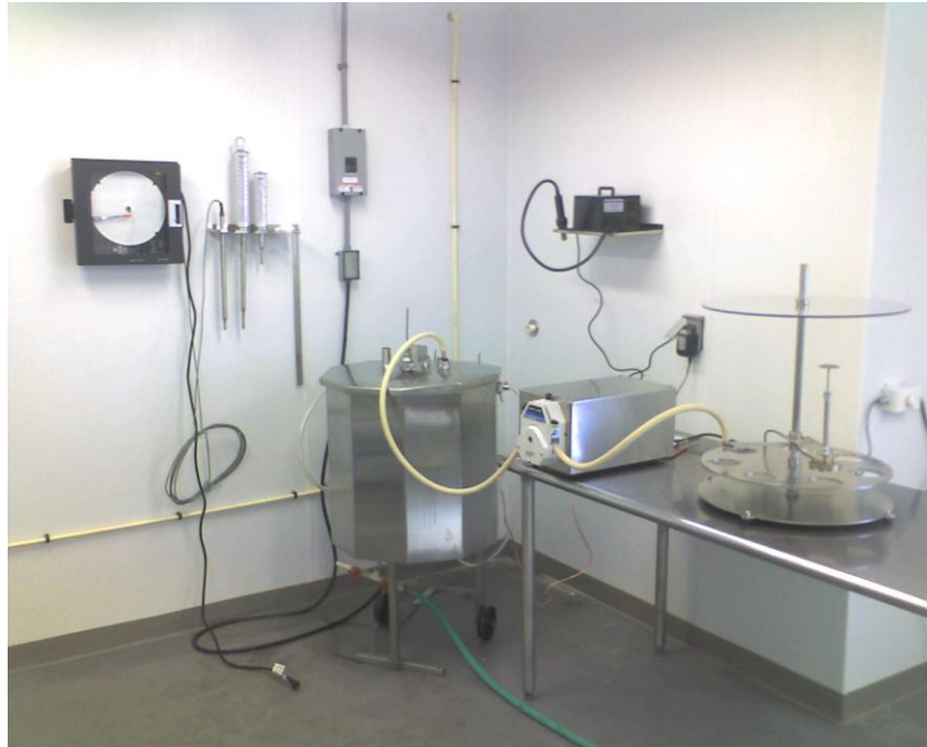
Typical Installation – Pasteurizer with Thermometers and Chart Recorder, Sanitary Tube Pump, Packager.
