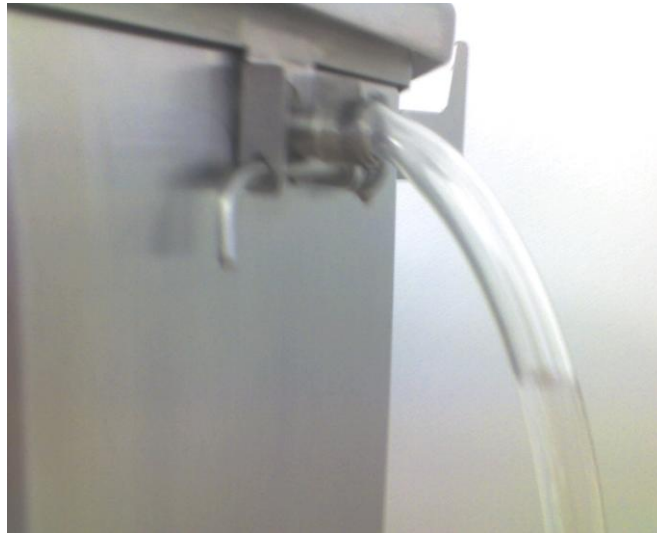
Sight gage to allow observation of water level in the water jacket. Pin locks product liner in position.
