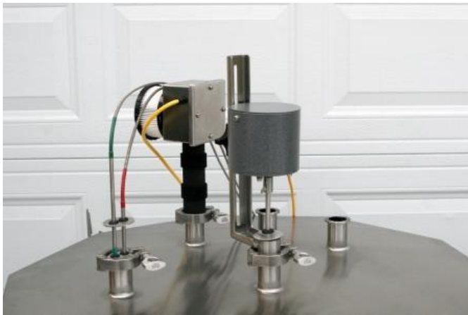
Pasteurizer lid (insulated). Ports included for airspace and product indicating thermometers, chart recorder probe, airspace heater, agitator and for filling/emptying the vat. Lid can be removed for manual cleaning.
