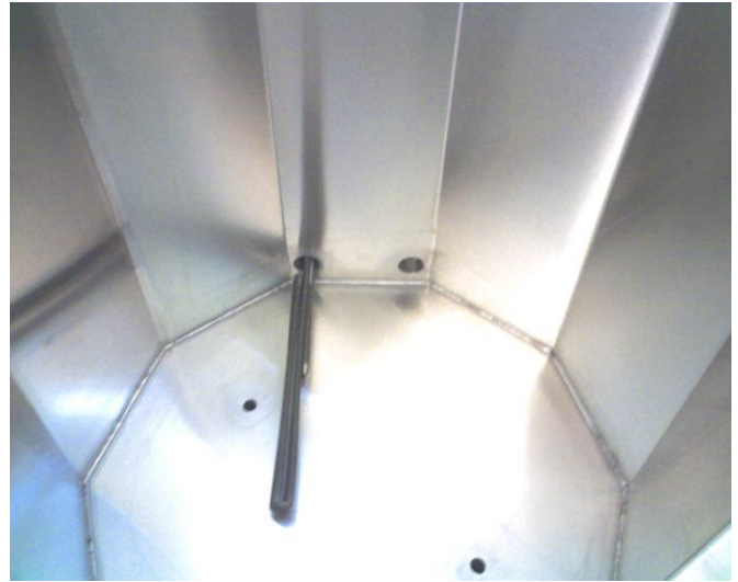
Pasteurizer with lid open to show water jacket and immersion heater in water jacket. Water Jacket is insulated.
