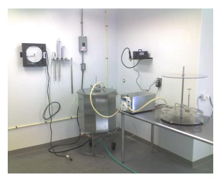
Typical Installation – Pasteurizer with Thermometers and Chart Recorder, Sanitary Tube Pump, Packager. Pasteurizer capacity – 2 to 22 gallons
