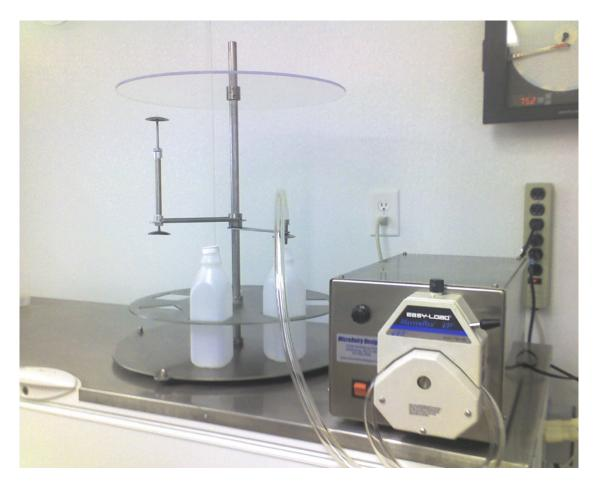
EcoFlex Packager showing sanitary shield, spring plunger for mechanical capping and sanitary tube pump for filling containers. The setup shown is for "snap cap" type plastic bottles. The packager can be set up to fill and cap glass and plastic bottles as well as "foil seal" yogurt cups and deli tubs. With the appropriate carriers, the packager can handle items as small as half-and-half creamers up to as large as gallon jugs. All containers are available with "tamper-evident" closures.
