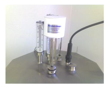
Agitator, Thermometers and Airspace Heater
