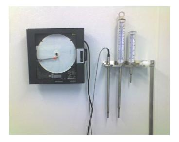
Chart recorder and probe, indicating thermometers
